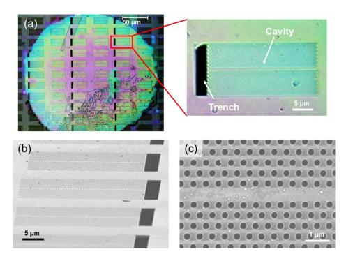
**Fig. 3.** (a) Optical microscope image of an array of fabricated PhC cavities on a thin diamond membrane window. Inset shows an enlarged microscope image of one of the PhC cavities. Scanning electron microscope images showing (b) angled and (c) top-down views of fabricated cavities. The image in (b) is taken at 75° stage tilt.
