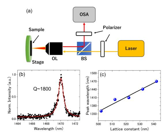
**Fig. 4.** (a) Illustration of the optical measurement setup. OL: objective lens; BS: beam splitter; OSA: optical spectrum analyzer. (b) Measured reflectance spectrum of the fabricated cavity with a = 542 nm (black squares), overlaid with a fit using a Lorentzian function (red curve). (c) Extracted cavity resonances by fitting (blue dots) as a function of lattice constant *a*. The black solid line shows the simulated resonance wavelengths by the FDTD calculations.
