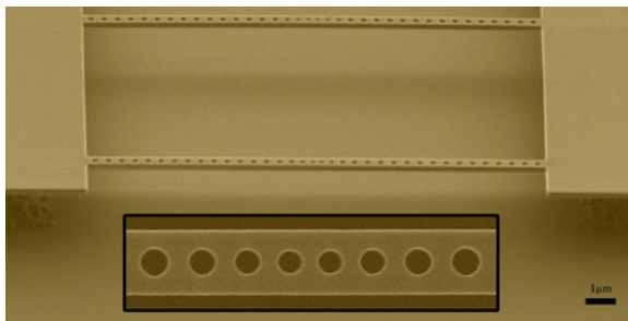
Photonic Crystal Nanobeam Cavities, Fig. 3 SEM image of the fabricated structure with a measured Q of 7.5 \times 10^5 [17]. The inset shows the zoomed cavity region
